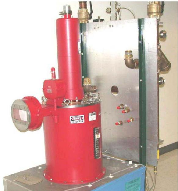
Figure 6: VKL-7966A Klystron in Electromagnet (Photo courtesy of TJNAF)
